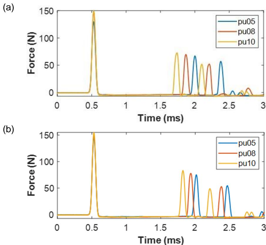
Fig. 2 Density Evaluation result according to thickness of PU foam covered with 0.5t(a)/2t(b) silicone layer
